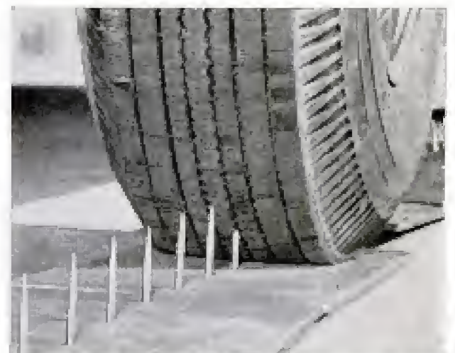
Pierced by spikes, BFG "Life-Saver" Tire loses no air
